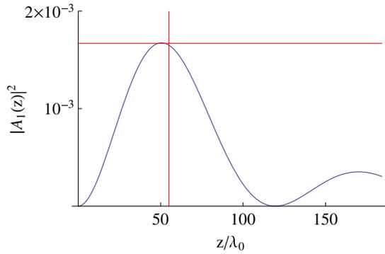
Fig. 4. Absolute square  $|A_1(z)|^2$  of the  $m = 1$  component of the exact solution (61) and the approximate coordinates (72), (73) of its first maximum. The parameters are chosen according to Table 1 and  $\theta_0 = (1/2)\theta_B$ .
