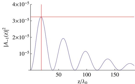
Fig. 5. Absolute square  $|A_{-1}(z)|^2$  of the  $m = -1$  component of the exact solution (61) and the approximate coordinates (72), (73) of its first maximum. The parameters are chosen according to Table 1 and  $\theta_0 = (1/2)\theta_B$ .
