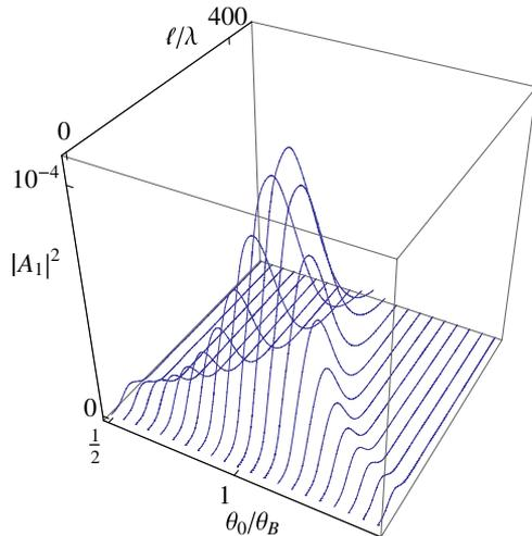
Fig. 2. Square amplitude  $|A_1|^2$  of the first diffraction order of the transmitted wave according to the exact solution of the diffraction problem and the values shown in Table 1. The two independent variables are the thickness of the crystal  $\ell$  in units of the wavelength  $\lambda_0$  and the angle  $\theta_0$  of the incident plane wave in units of the Bragg angle  $\theta_B$ .
