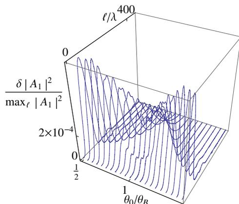
Fig. 3. Difference  $\delta|A_1|^2$  between the square amplitudes of the exact solution according to Fig. 2 and those of the corresponding CWT divided by the maximum of  $|A_1|^2$  w. r. t.  $\ell$  and fixed  $\theta_0$ . The independent variables are the same as in Fig. 2. Note that the relative difference increases with the deviation of  $\theta_0$  from the Bragg angle but never exceeds  $10^{-3}$ .
